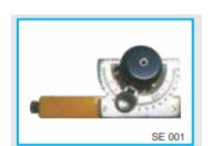
Telescopicwithdoubledrawtube& slowmotionarrangementArcdividedto 30 min.& readingbyvernierto 10min.
