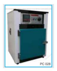
Double walled, Outer chamber made of M.S. Powder Coated. Temp. upto 250deg C. Thermostatic controlled, Heating Element on three sides. Thermometer is provided on top. The scale is calibrated in 5 deg C Steps
