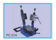
operated semi automatic machine for various operations. (I) Plates for putting of capsules. (ii) Removal of caps (iii) Filling of powder by dispensing brush, pressing (iv) Ejection of 100 capsules of 0,00,1, 2, or 3 Any one size on order)
