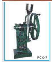
SINGLE PUNCH for making Tablets up to 1000 mg as per size of die & punch 6, 9 & 12 mm (Any one). Automatic compression & ejection device with each revolution of the wheel drive. Built on heavy cast iron body with eccentric pressure system. Stainless steel hopper provided & connected by a Rubber tube. Easy setting for thickness & hardness of tablets with lock nuts. Die & set of punches are chromium steel.
