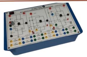
panels are RESISTANCE CAPACITORS IC Ne555 VARIABLE RESISTOR 10K PULSAR SWITCH SALIENT FEATURES: Front panel built with high class insulated Printed Circuit Board sheet with well printed circuits and symbols. Fuse for Short Circuit protection Instruction manual. Connections are brought out through 2mm Colored Sockets. Patch Cords 2mm.
