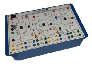
**AGN-067A Description :** 555 Timer as Astable Multivibrator Apparatus has been designed to study the Wave Shape and Frequency produced by Astable Multivibrator. IC 555 placed inside the cabinet & connections brought out at sockets. DC regulated power supply of 5V. Various resistances & capacitors connected inside the cabinet & connections brought out at the sockets.
