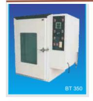
(Inner S.S) Temp 5 deg C above ambient to 60 deg C. Humidity 30-90%
