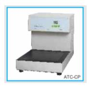
It is used to cool specimen blocks. The temperature can be easily set through the feather touch keys and it also has a memory to store the pre-used temperature. The large plate can easily accommodate upto 50-80 cassettes. Technical Specifications
