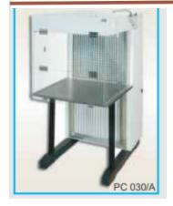
Structure made of times ply board with summed from outside & S.S. Workbench. Clear acrylic side panels & front door. HEPA Filter efficiency 99.97% upto 0.3 micron.
