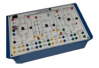
AGN-067A Description: 555 Timer as Astable Multivibrator Apparatus has been designed to study the Wave Shape and Frequency produced by Astable Multivibrator. IC 555 placed inside the cabinet & connections brought out at sockets. DC regulated power supply of 5V. Various resistances & capacitors connected inside the cabinet & connections brought out at the sockets.
