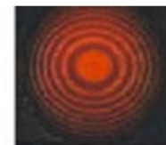
Fringes of Michelson Interferometer with He-Ne laser.
