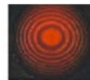
Fringes of Michelson Interferometer with He-Ne laser.
