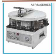
ונ וז ממשבע טוו אווו עא נווווכו וטו אוטקומווווווווון מטנוו עכומץ and processing cycle and no need of cutting plier for programming. Technical Specification Number of stations: 12 Reagent Stations: 10 Paraffin Wax Bath(Station): 2 Delay Start: upto 24hrs Safety Device: Yes Basket Rotation: Yes (4 R.P.M.) Supplied complete as above with 10 reagent beakers, 2 wax bath thermostatically controlled, 24 S.S Tissue Cassettes , 1 S.S. Basket, dust cover and operational manual.
