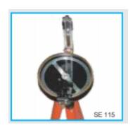
Made of Brass & Aluminium floating circle graduated to read 30mins. An automatic lifter along with reflecting mirror is fitted on sight vane. Packed in sling case.
