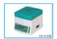
MICRO CENTRIFUGE MACHINE (Digital), T-12 Microprocessor speed control, LCD R.P.M,Timer 0-59min, Max 13000rpm in steps of 100rpm (with load). Supplied With 12x1.5 / 2ml Rotor Head & heavy plastic injection moulded body.
