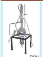
Automatic Electrically Heated All Glass Distillation Unit, NPL Design, Heater Embedded In Spiral Glass Tube Complete With Heavy Base, Rod, Clamps, Boards Etc. Read More
