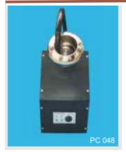
operated independently & air is thermostatically controlled to give temperature 30 to 110 degrees. Switches for motor, blower, heater and Thermostat are fixed on a panel with neon indicators. Also mains lead with 15 amps plug provided.
