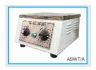
It is rectangular in shape and used to heat slides at a uniform temperature just below the melting point of wax so as to provide flattening without any damage to the section. The top plate is securely mounted on a insulated metal base. Technical Specifications Temperature Range : ambient to 90 Degree ● Hot Plate Dimensions (Inch): 12x10 Supplied complete with cord and plug and is suitable to work on 220/230V-AC Supply
