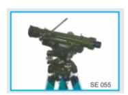
Internal Focusing, Showing Inverted Image as per IS specification with Aluminium Folding Stand Read More
