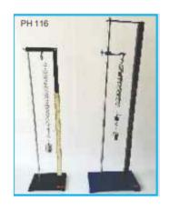
APPARATUS "AGN Make With Spiral Spring About 25mm Dia & 10cm Long On Metal Base With 250gm Slotted Weight. Heavy Pattern with Graduated Metal Pipe (Superior)
