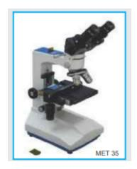
Fixed Stage 120x130mm with Detachable Mechanical Stage. Smooth Lever type Fine Motion Focusing, Quadruple Revolving Turret Nose Piece with Click Stops. Achromatic Objectives M 10x & M 40x. Eyepiece WF 10x. Incident Light through 20 W Halogen Lamp with iris Diaphragm & Filter Slots.
