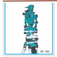
Direct Neading, Size 17311111 (7 ), L.C. 20 Second, With Optical Plummet & blue coated optics showing erect image circles. Internal Focusing with Aluminium Stand & Accessories in wooden box.
