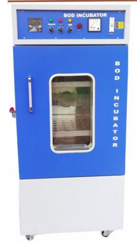
repeat from 1 - 98 times or unlimited programmed operations and Minimum 10 programs memorized \* CFC-free Foamed-in-place Rigid Polyurethane Insulator & Hermetic Compressor \* Triple-pane Glass Observation Window plus 15W Fluorescent Lamp \* Independent Over-Temp. Protection Device isolated from main circuit \* Programmed Memory Backup & Automatic Return Buzzer Switch
