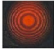
Fringes of Michelson Interferometer with He-Ne laser.
