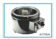
This circular floatation bath is ideally suited for preparing of distortion less and wrinkle free tissue specimens. It is a double walled unit with inside made up of aluminum and outside MS sheet which is duly painted. Technical Specifications
