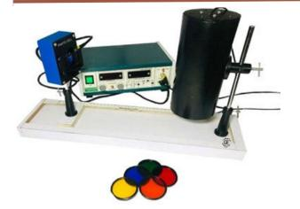
M-200 Description : Experimental Set-up has been designed specifically for determination of Planck's constant by Vacuum type Photo Cell with three ilters. The experimental set-up is absolutely self contained and require no other apparatus. Photo Cell with three ilters. Practical experience on this set up carries great educative value for Science and Engineering Students.
