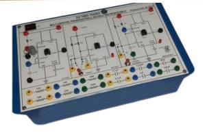
panels are RESISTANCE CAPACITORS IC Ne555 VARIABLE RESISTOR 10K PULSAR SWITCH SALIENT FEATURES: Front panel built with high class insulated Printed Circuit Board sheet with well printed circuits and symbols. Fuse for Short Circuit protection Instruction manual. Connections are brought out through 2mm Colored Sockets. Patch Cords 2mm.
