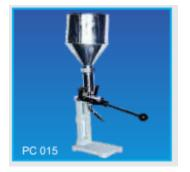
Stroke type, barrel and piston arrangement with stroke setting for various capacity of filling tubes detachablenozzles provided for each separate capacity. All contact parts are Brass. Built on cast iron body. Cap. 5gm to 50gm
