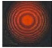
Fringes of Michelson Interferometer with He-Ne laser.
