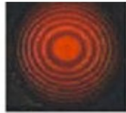
Fringes of Michelson Interferometer with He-Ne laser.
