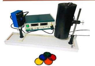
M-200 Description : Experimental Set-up has been designed specifically for determination of Planck's constant by Vacuum type Photo Cell with three ilters. The experimental set-up is absolutely self contained and require no other apparatus. Photo Cell with three ilters. Practical experience on this set up carries great
