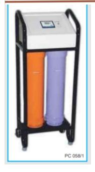
Capacity Jo Eti/iii , Colisists of two plastic coluitiii charged with high exchange capacity Cation & Anion resins. Conductivity Meter Provided
