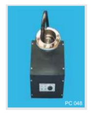
12" Dia stainless steel, the machine worked by oil immersed gearbox, with F.H Motor drive. Air blower is operated independently & air is thermostatically controlled to give temperature 30 to 110 degrees. Switches for motor, blower, heater and Thermostat are fixed on a panel with neon indicators. Also mains lead with 15 amps plug provided.
