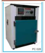
Double walled, Outer chamber made of M.S. Powder Coated. Temp. upto 250deg C. Thermostatic controlled, Heating Element on three sides. Thermometer is provided on top. The scale is calibrated in 5 deg C Steps
