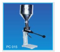
Stroke type, barrel and piston arrangement with stroke setting for various capacity of filling tubes detachablenozzles provided for each separate capacity. All contact parts are Brass. Built on cast iron body. Cap. 5gm to 50gm
