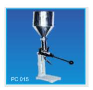
Stroke type, barrel and piston arrangement with stroke setting for various capacity of filling tubes detachablenozzles provided for each separate capacity. All contact parts are Brass. Built on cast iron body. Cap. 5gm to 50gm
