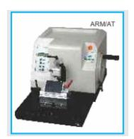
movement and high precision motorized specimen feed, for high throughput histology labs. Powerful sectioning motor enable us to cut even the hard specimen easily. The smartly located feature keypad enables us to control the operation easily. Apart from other safety feature it also has an emergency stop button. **Salient Features** • LCD Display to indicate section Alarm to indicate start/end of travel Motorized forward and backward at ● Adjustable specimen retraction
