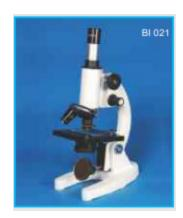
15x & two objectives 10x, 45x, with fixed condenser AGN Make (KG-2) 'ISI Marked' (In Wooden Box)
