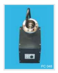
immersed gearbox, with F.H Motor drive. Air blower is operated independently & air is thermostatically controlled to give temperature 30 to 110 degrees. Switches for motor, blower, heater and Thermostat are fixed on a panel with neon indicators. Also mains lead with 15 amps plug provided.
