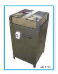
Determines Hardenability of Steel. Muffle Furnace can be purchased extra for the complete Experiment.
