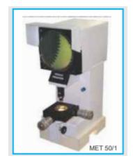
Rotatable 360 deg with 2 min Vernier Resolution.
