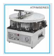
It is based on pin up timer for programming both delay and processing cycle and no need of cutting plier for programming. Technical Specification Number of stations: 12 Reagent Stations: 10 Paraffin Wax Bath(Station): 2 Delay Start: upto 24hrs Safety Device: Yes Basket Rotation: Yes (4 R.P.M.) Supplied complete as above with 10 reagent beakers, 2 wax bath thermostatically controlled, 24 S.S Tissue Cassettes ,1 S.S. Basket, dust cover and operational manual.
