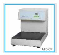
can be easily set through the feather touch keys and it also has a memory to store the pre-used temperature. The large plate can easily accommodate upto 50-80 cassettes. Technical Specifications • Capacity: 60-80 Cassettes ● Overall Dimensions (mm): 640x370x410 Read More
