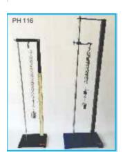
**Spiral Spring About 25mm Dia &** 10cm Long On Metal Base With 250gm Slotted Weight. Heavy **Pattern with Graduated Metal Pipe (Superior)**
